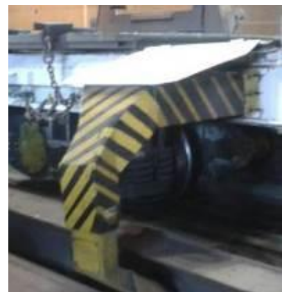
Marking of moving and protruding elements of equipment, shelter and barriers.
